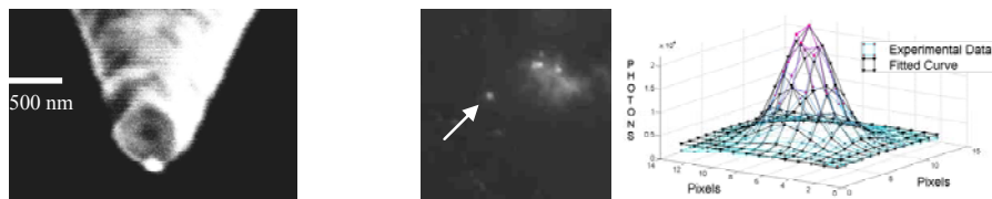
Fig.2. Left: Metal coated probe, with an aperture at the apex, fabricated at the PI's laboratory. Right: Image of spread fluorophore markers captured by our CCD camera. The arrow indicates the point-source chosen for the Gaussian function fitting algorithm (from preliminary work currently being performed at the PI's laboratory.)
